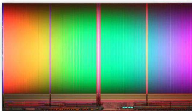
Figure 4. Intel Micron 8 GB NAND flash device, 2 bit per cell, 25 nm minimum feature, 16.5 mm x 10.1 mm [5].
