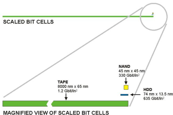
Figure 1. Scaled views of YE2010 bit cells for NAND, HDD, and TAPE
